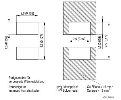
For superior solder joint connectivity results we recommend soldering under standard nitrogen atmosphere. Package not suitable for ultra sonic cleaning.
